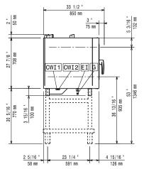
C- = Cold W WI- (cleaning) Cold Water inlet 1 ΕI Electrical inlet (power)
